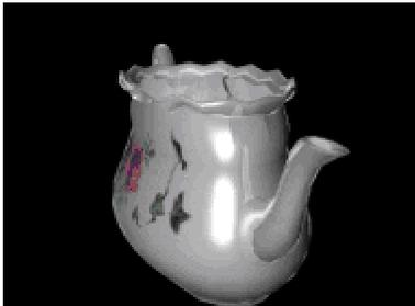
**Color Plate 2:** The screen snapshot shows specular reflection on the surface of the teapot. Notice that the reflected highlights are the color of the incident light, not that of the surface material (see [Chapter 4](#) for more information). The teapot in this example is a model for nonperfect reflectors as described by Phong Bui-Tuong.
