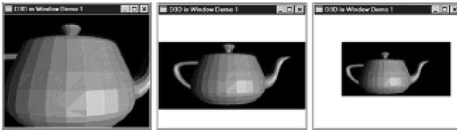
**Figure 15-1:** Effect of changing the camera position along the z-axis
